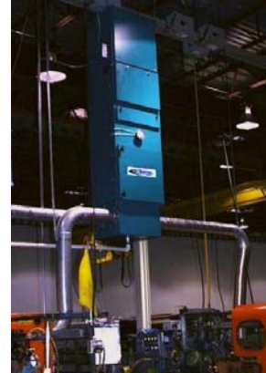
FVDH-30-05S system with special filters for control of dust, light mist and smoke from cast iron machining.
