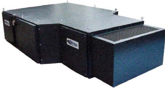
Custom FHDC2-90-60SXP with special prefilters, direct drive explosion proof high pressure blower and upblast attenuator for control of paint overspray and vapors.
